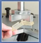
Enables a quick change to a different clamping pad depending on joining applications
